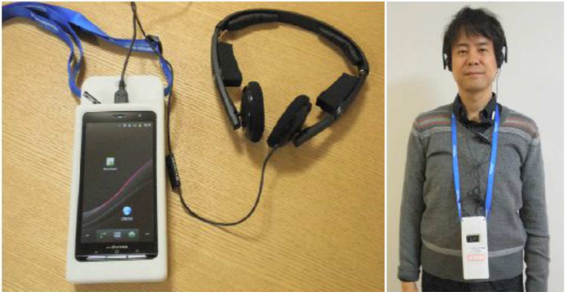
VLC detector with Magnetic field sensor. Audio guide is given by its headphone. Panasonic and Keio Univ. experiment system.
