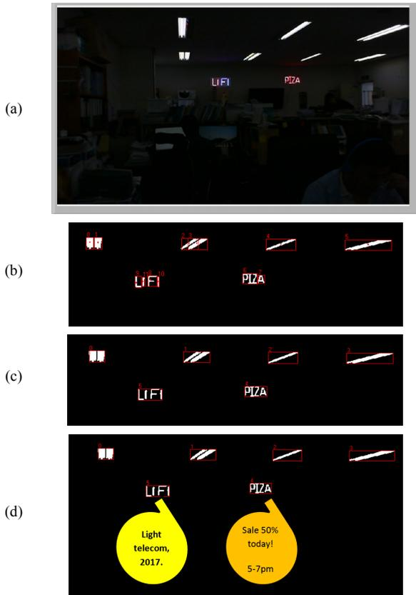
**Fig-4. The processing procedure of textured-LED at a receiver** (a) An image of textured-LED captured at 7m distance, (b) The detection of light sources, (c) Grouping LEDs and RoIs defining, (d) Data reception from the signaling RoIs.
