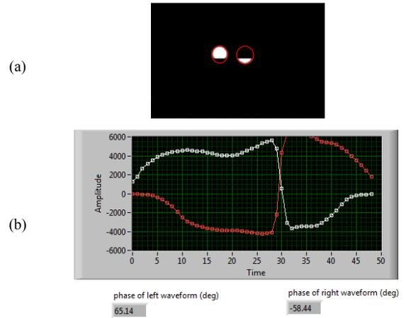
**Fig-5. The waveforms extracted from a pair of LEDs** (a) LED bulbs, (b) Waveforms extracted from LEDs.
