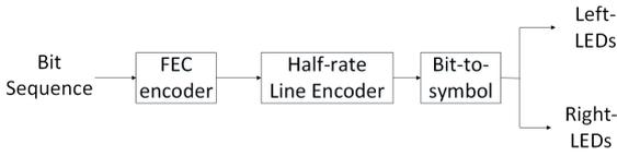
Fig-2. Reference architecture for S2-PSK transmitter
