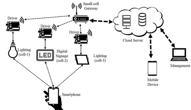
Fig-1. Overall architecture of OCC Small-Cell
