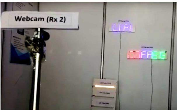
Fig-3. A demo of OCC using textured-LEDs and LED tube
